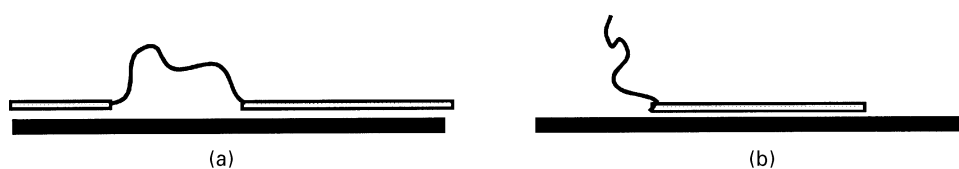
Fig. 1. Schematic diagrams, based on predictions of self-consistent-field calculations, depicting typical conformations of (a) \alpha_{s1} -casein and (b) \beta -casein adsorbed onto planar hydrophobic interface. Bars are simply used to denote hydrophobic regions of molecules and do not imply rigidity.
