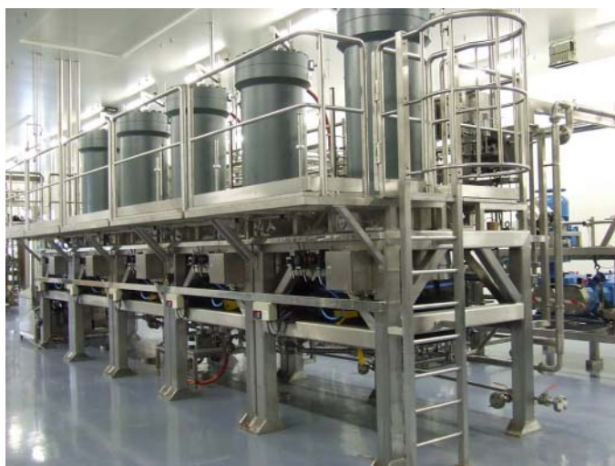
Figure 10.22 Varicol multicolumn (1 m i.d.) continuous process. Source: Reproduced with permission of NOVASEP.
