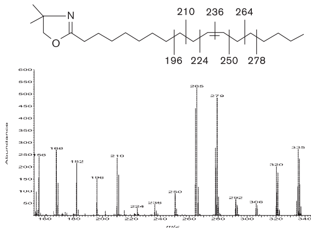
Fig. 4. Mass spectrum of 4,4-dimethyloxazoline derivative of VA produced from LA by Ros. inulinovorans . Relative abundance of ion fragments at m/z 210 and 211 indicates that ^2\text{H} is located on C-9 of the fatty acid moiety. Comparison of ion fragments at m/z 264, 265 and 266 reveals additional enrichment of ^2\text{H} on C-13 of the fatty acid moiety. Bu. fibrisolvens , Ros. hominis and Rum. obeum gave similar spectra.
