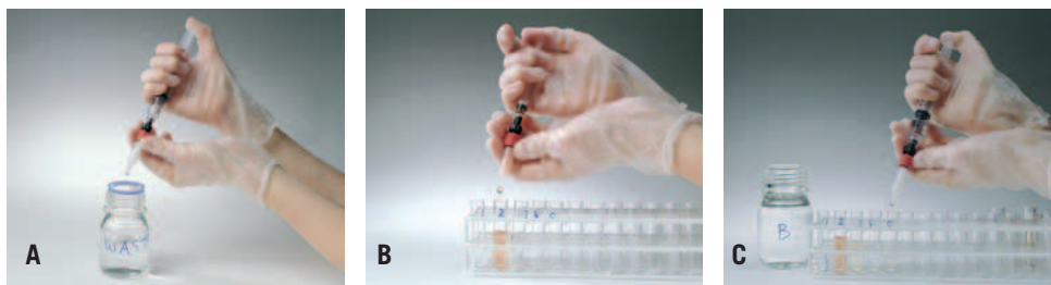
Fig. 24. Using GSTrap FF with a syringe. A: Prepare buffers and sample. Remove the column's top cap and twist off the end. B: Equilibrate column, load the sample and begin collecting fractions. C: Wash and elute, continuing to collect fractions.
