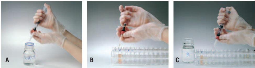
Fig. 16. Using HiTrap Protein G HP with a syringe. A: Dilute buffers and prepare sample. Remove the column's top cap and twist off the end. B: Equilibrate the column, load the sample and begin collecting fractions. C: Wash and elute, continuing to collect fractions.
